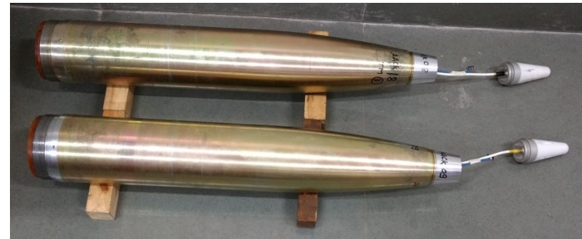
Monopole antenna for Rocket with metallic ogive
